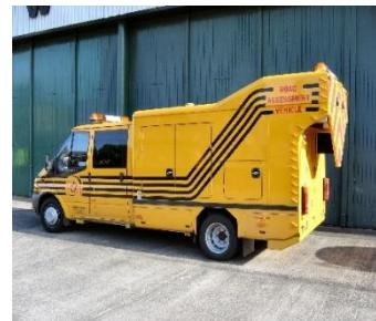
The condition of principal and non-principal networks is assessed annually through SCANNER surveys. These traffic-speed, machine-based surveys measure various road condition parameters, which are processed in the pavement management system (PMS) to create a road condition indicator (RCI) for every 10-metre sub-section.
