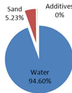
2.6.6 Additives in the water include surfactants to enable the fluid to pass easily through fractures, bactericides and acids to prevent build-up of scale in the well. All chemical additives used in hydraulic fracturing require pre-approval by the Environment Agency and are required to be non-hazardous (non-carcinogenic)
