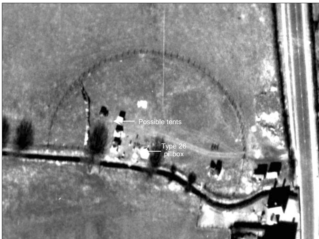
Figure 37. A previously unrecorded pillbox, type FW3/26 at Longford (NRHE: 1583785), with nearby tents and a fenced off perimeter. NMR RAF/106G/UK/1293 RV 6023 25-MAR-1946 Historic England RAF Photography
