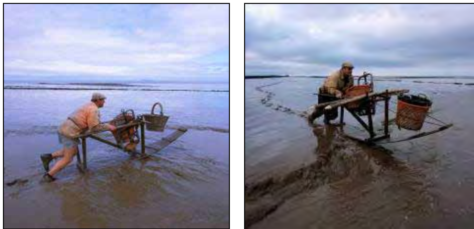
Figure 5.34. Adrian Sellick pushing his mudhorse across the thick wet mud. The wooden sled and its runners spreads the weight of the fisherman and his catch, enabling him to travel across the mud.
