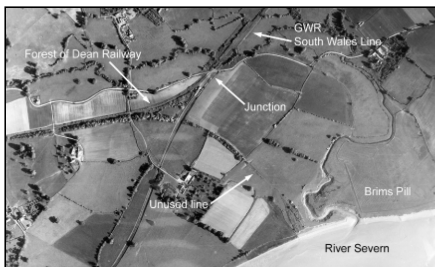
Figure 9.45. The junction of the Forest of Dean Railway with the GWR South Wales Line and the unused line to Brims Pill (taken from Forest of Dean RCZAS survey).
