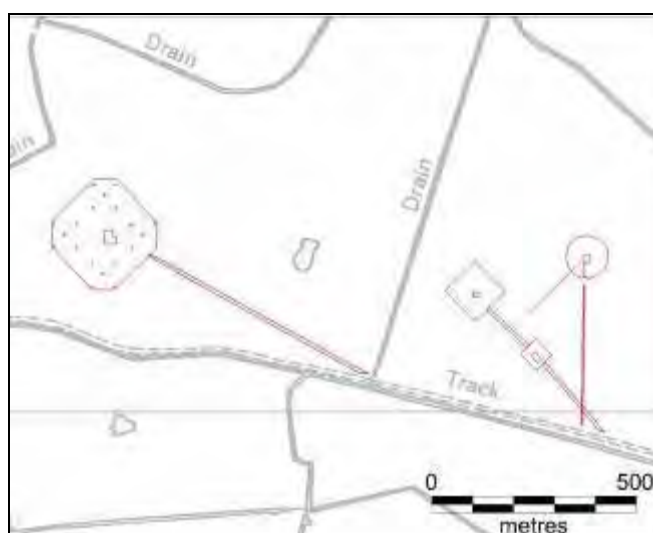
Figure 10.27. The Second World War maritime radio receiving station near Burnham-on-Sea. The antennas are shown enclosed by fences (purple). Trackways have also been recorded extending from the individual sites.
