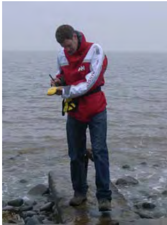
Plate 1: Nick Witchell of GCCAS using the Trimble GeoXT and Geobeacon to record a feature (a concrete base) at Lilstock Harbour, Somerset.
